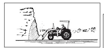
Exercise caution when undercutting high banks. Dirt slides can be dangerous. Load from as low as possible for maximum efficiency. Loader lift and breakaway capacity diminish as loading height is increased.
